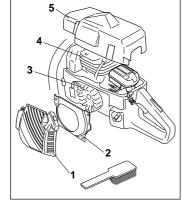
Clean the cooling system with a brush once a week, more often in demanding conditions. A dirty or blocked cooling system results in the saw overheating which causes damage to piston and cylinder. NOTE! The cooling system of chain saws that are fitted with a catalytic converter must be cleaned daily. This is particularly important on saws with catalytic converters, because the higher working temperature of the exhaust demands efficient cooling of the engine and the catalytic converter unit.
